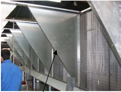
Economizer, increase 15% of capacity, with less energy (optional)
